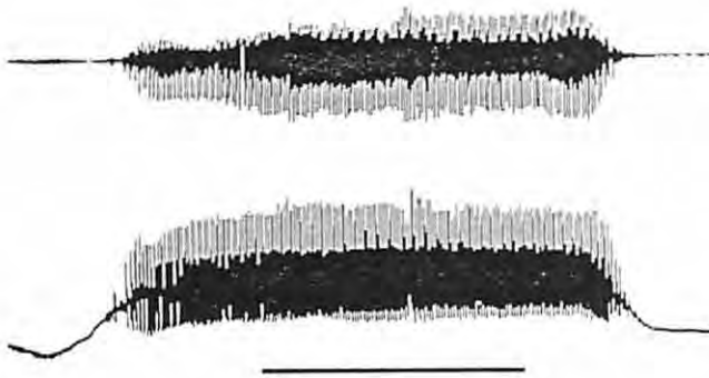
Figure 1. Example of a vocalization categorized as a growl from Dog 6. The top trace is the acoustic signal and the bottom trace is tracheal pressure ( P_t ). The fundamental frequency ( F_0 ) of the vocalization was determined by spectral analysis to be 112 Hz. The portion of the P_t signal to be measured in this example is indicated by the bar (0.8 s) beneath the data. Average P_t in this example is 2.9 kPa.
